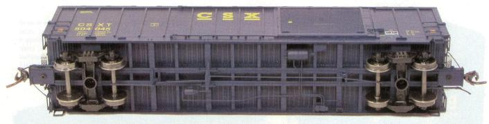
The car's underframe reveals cleanly assembled superb floor and brake rigging details. The relief valve on the side sill is seldom seen on a model, as is the standoff door track. A door that slides
